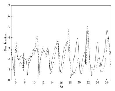
Figure 5. Form functions of two stainless-steel spheres immersed in water at broadside incidence ( $\alpha = \pi/2$ ) versus ka for the separation distance d = 2a: —, theory; –, experiment.
