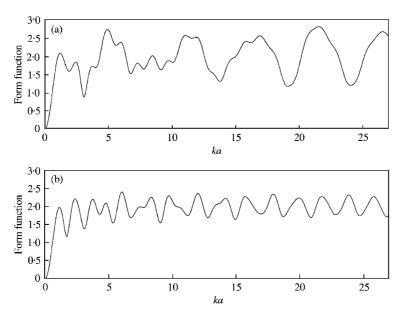
Figure 3. Computed form functions of two rigid spheres at broadside incidence ( $\alpha = \pi/2$ ) versus ka for the separation distances: (a) d = 2a, (b) d = 4a.
