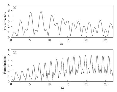
Figure 2. Computed form functions of two rigid spheres at end-on incidence ( $\alpha = 0$ ) versus ka for the separation distances: (a) d = 2a, (b) d = 4a.
