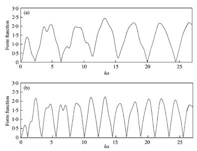
Figure 4. Computed form functions of two rigid spheres at oblique incidence ( $\alpha = \pi/4$ ) versus ka for the separation distances: (a) d = 2a, (b) d = 4a.
