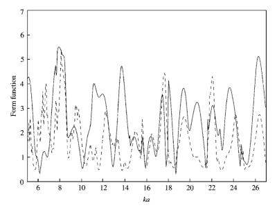
Figure 7. Form functions of two stainless-steel spheres immersed in water at end-on incidence ( $\alpha = 0$ ) versus ka for the separation distance d = 2a: —, theory; –, experiment.
