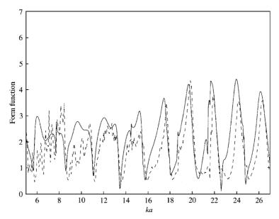
Figure 6. Form functions of two stainless-steel spheres immersed in water at broadside incidence ( $\alpha = \pi/2$ ) versus ka for the separation distance d = 4a: —, theory; –, experiment.
